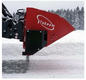
Self-loading spreader built as a bucket. SMA is used for spreading sand, salt or grit. The spreading material is distributed by a feeding auger. Its quantity is determinated by the speed of auger
