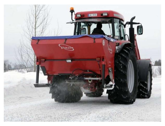
Used for spreading of large open areas as well as roads. The quantity of material and the spreading width are adjusted independently (by the hydraulic flow regulator on the spreader). The spreading symmetry can be adjusted hydraulically (controlled by the hydraulic flow from the tractor cabin).
